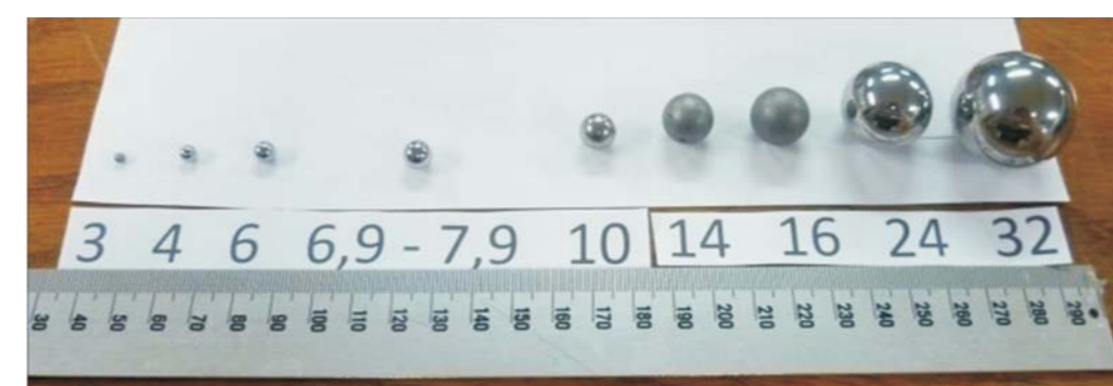
Size of abrasive material in abrasion regime R1
